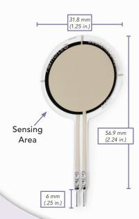
The FlexiForce A401 is our standard piezoresistive force sensor with the largest sensing area. It is available off-the-shelf for easy proof of concept and is also available in large volumes for design-in applications. The A401 sensor has a 2-pin connector and is designed to use with your own electronics or multimeter.
