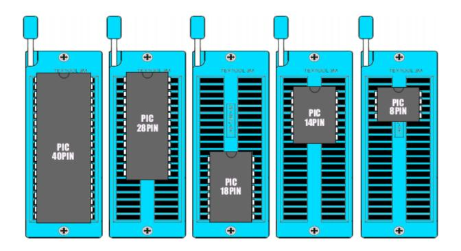
The IC should be placed in the ZIF socket as shown in the diagram.
