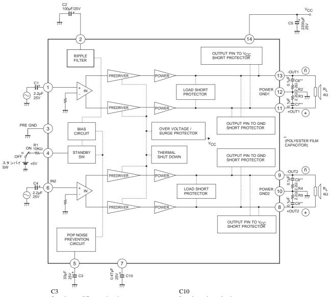
Sets the amplifier starting time (Approximately 0.6 seconds when  $33\mu$ F)
