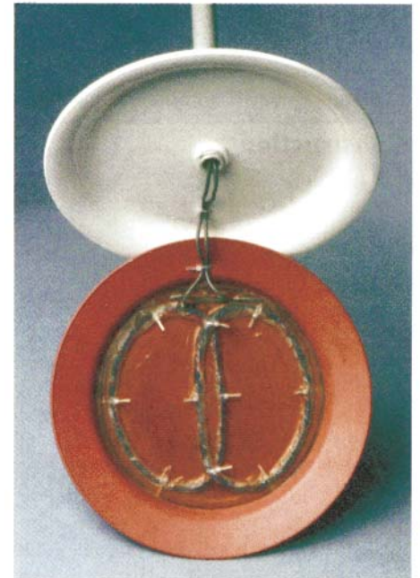
This photo clearly shows the potted search coils in situ.
