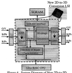
Figure 4. System Diagram of New 2D-to-3D Conversion LSI and Peripherals
