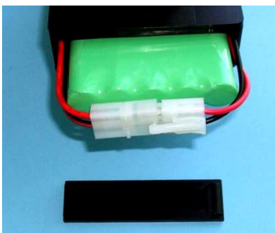
Carefully Pull out the Battery
