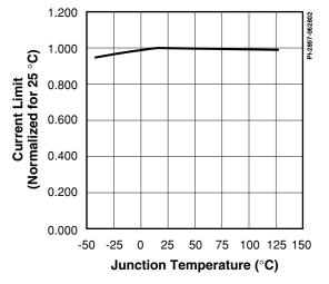
Figure 19. Current Limit vs. Temperature.
