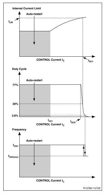
Figure 4. CONTROL Characteristics.
