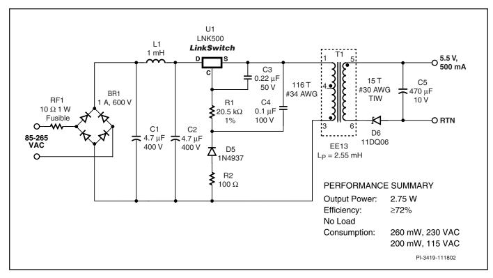
Figure 9. 2.75 W Constant Voltage/Constant Current (CV/CC) Charger using LinkSwitch.
