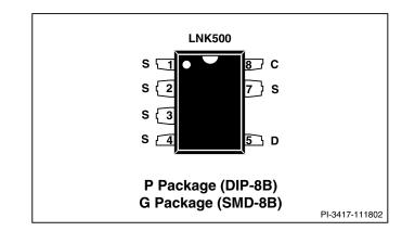
Figure 3. Pin Configuration.
