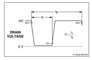
Figure 14. Duty Cycle Measurement.
