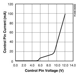
Figure 15. CONTROL Pin I-V Characteristic.
