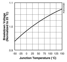
Figure 17. Breakdown Voltage vs. Temperature.
