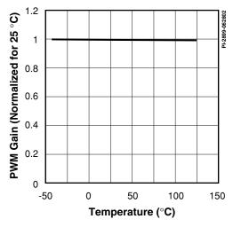
Figure 22. PWM Gain vs. Temperature.
