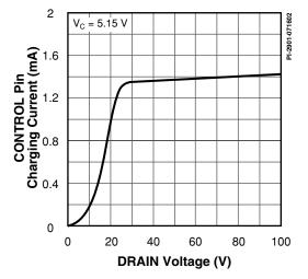
Figure 13. I<sub>c</sub> vs. DRAIN Voltage.
