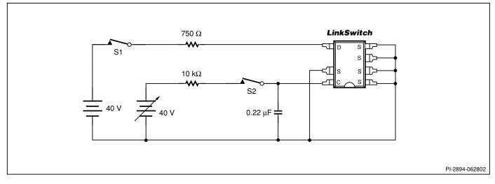
Figure 12. LinkSwitch General Test Circuit.
