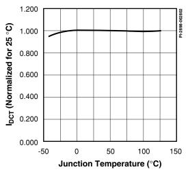
Figure 21.  $I_{DCT}$  vs. Temperature.
