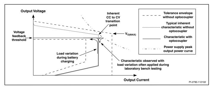
Figure 8. Output Characteristic with Optocoupler Regulation (Reduced Voltage Feedback Threshold).
