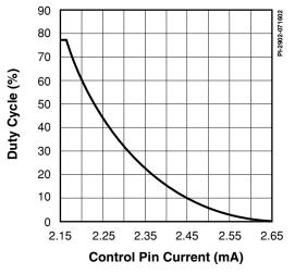
Figure 16. Duty Cycle vs. CONTROL Pin Current.
