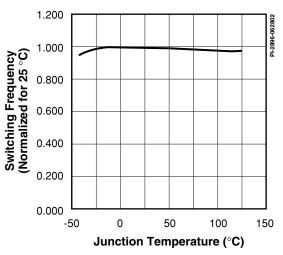
Figure 18. Switching Frequency vs. Temperature.
