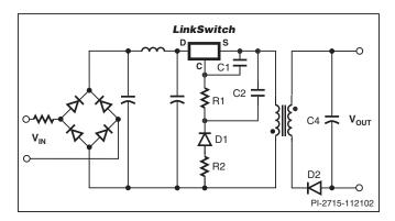
Figure 5. Power Supply Outline Schematic.
