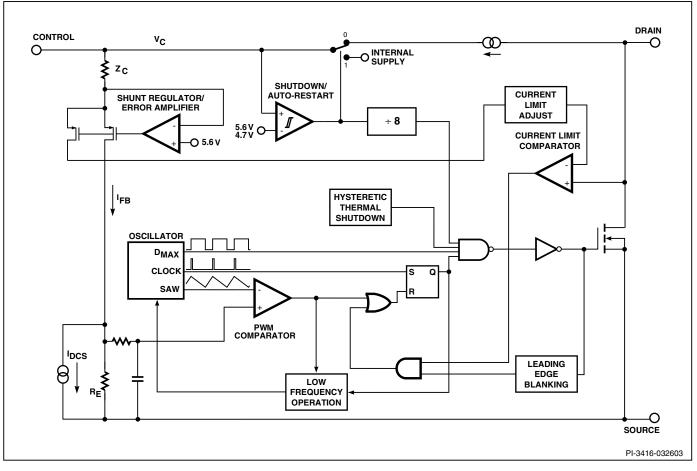
Figure 2. Block Diagram.
