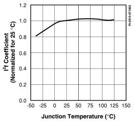
Figure 20. I'f Coefficient vs. Temperature.
