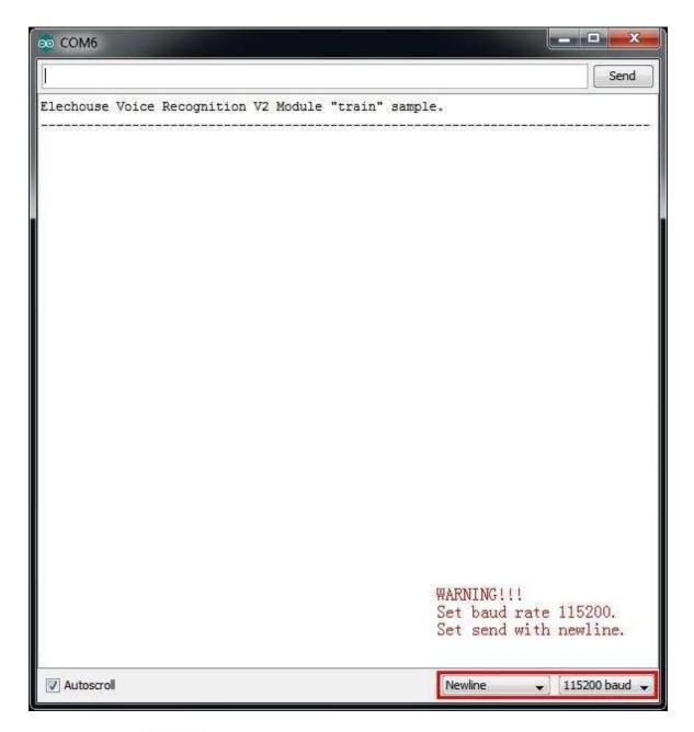
5. Send command settings(case insensitive) to check Voice Recognition Module settings. Input settings, and hit Enter to send.
